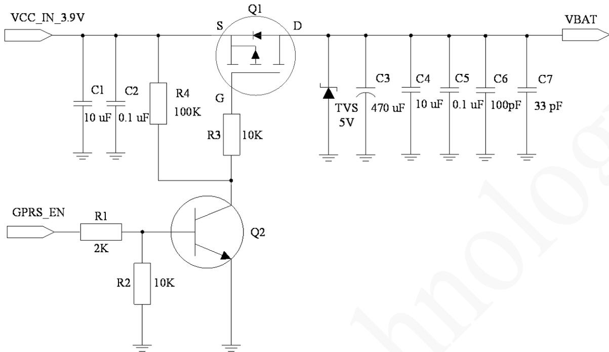
Q2 is added to eliminate the need for a high enough voltage level of the host GPIO. In case that the GPIO can output a high voltage greater than  $VCC\_IN\_3.9V - |V_{GS(th)}|$ , where  $V_{GS(th)}$  is the Gate Threshold Voltage, Q2 is not needed.
