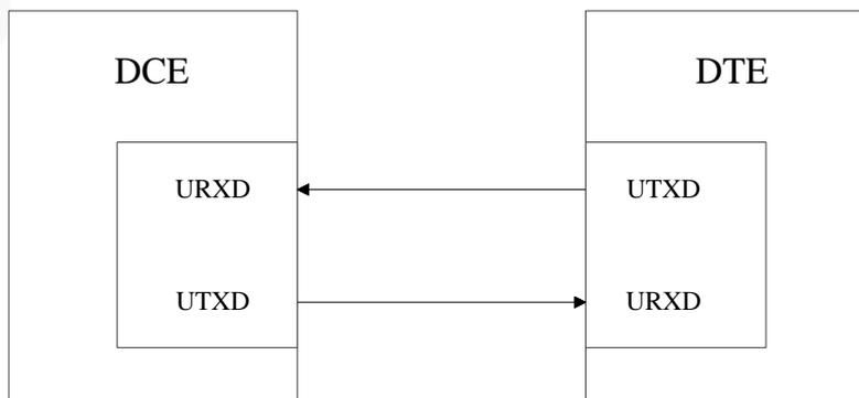
The UART of M590E V1 works at **2.8 V** CMOS logic level. The voltages for input high level should **not** exceed 3.1 V. Supported baud rates are 9600, 14400, 19200, 38400, 57600, 115200 bit/s, and the default rate is **115200 bit/s**.
