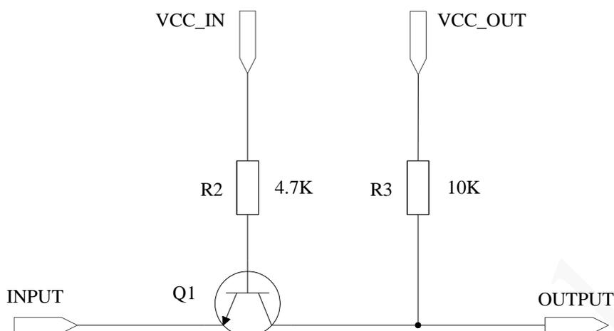
In Figure 3-13, INPUT is connected to UTXD of the MCU and VCC\_IN is connected to the 5 V power supply of the MCU. OUTPUT is connected to URXD of the module and VCC\_OUT is connected to VDD\_EXT(2.8V) of the module. If the circuit is far away from the VDD\_EXT pin, add a 0.1  $\mu$ F decoupling capacitor to VCC\_OUT.
