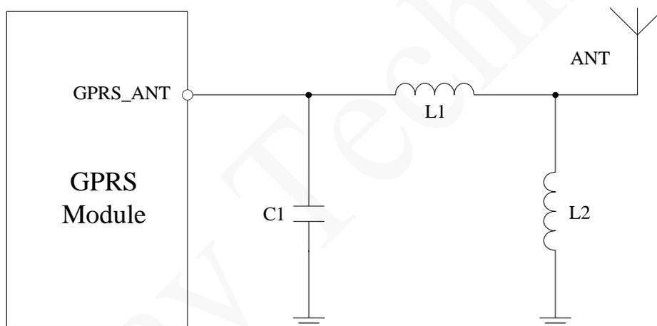
On two-layer boards which cannot control resistance properly, the RF route should be as short and smooth as possible and at a width of 1 mm; the RF is 1 mm away from the ground.
