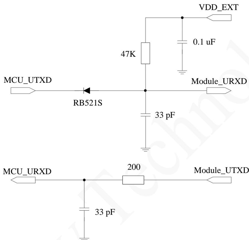
In Figure 3-12, 100 pF filter capacitor should be placed near the receive pin of the module. Resistance (200  $\Omega$  to 470  $\Omega$ ) and capacity (100 pF to 470 pF) can be selected based on the tested signal wave. Great serial resistance and filter capacity will decrease the signal level, resulting in great signal wave distortion and the low adaptable UART communication baudrate. RB521S-30TE-61, RB521SM-30GJT2R, and LRB521S-30T1G are recommended for separating diode.
