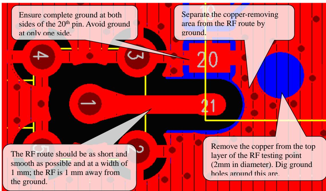
If you use RF feeder to connect the module and the antenna (pin 21 is not used), remove the pad of the 21<sup>st</sup> pin and its adjuncts. Refer to Figure 3-20.
