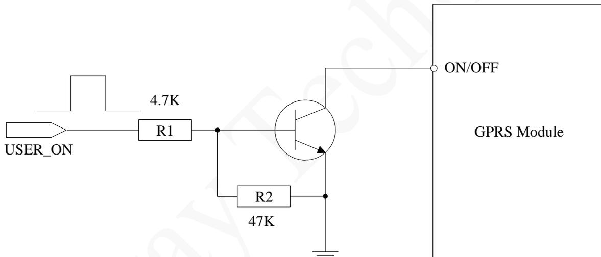
In Figure 3-9, high level takes effect for **ON/OFF** on the user side (USER\_ON) after level shifting.
