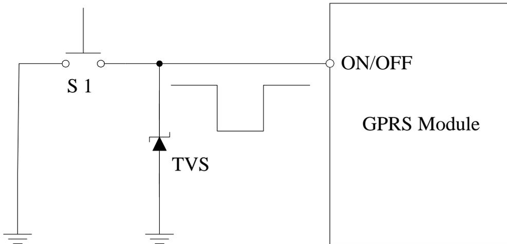
Figure 3-9 Reference circuit for power-on/off controlled by high level
