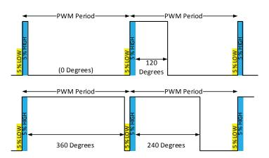
Figure 3: Pulse-Width Modulation (PWM) Examples
