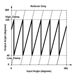
Figure 16: CE = 1, ROE = 0. Applied gain =  $4\times$ . LOW\_CLAMP = 10 ( $\approx$ 40°), HIGH\_CLAMP = 10 ( $\approx$ 320°)
