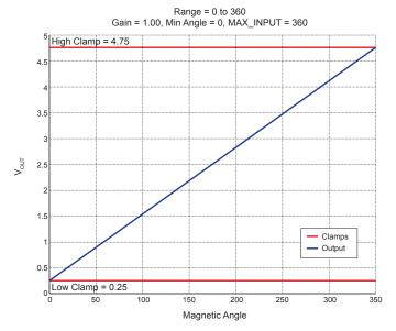
**Figure 18: Scenario A.**Regular output for a 0-360 degree input angle.
