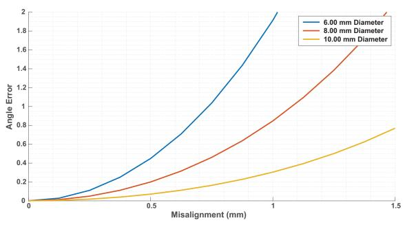
Figure 28: Simulated Error versus Eccentricity for different size magnet diameters, at 2.0 mm air gap
