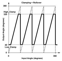
Figure 17: CE = 1, ROE = 1. Applied gain = 4×. LOW\_CLAMP = 10 (≈40°), HIGH\_CLAMP = 10 (≈320°)
