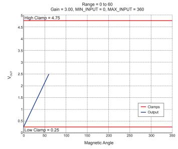
**Figure 21: Scenario D.** 0-60 degree input. Gain = 3. With an increased Gain value of  $3\times$ , the same 60-degree input signal now results in 50% of  $V_{CC}$ . The output signal is still free to swing from 5% to 95% of  $V_{CC}$ .
