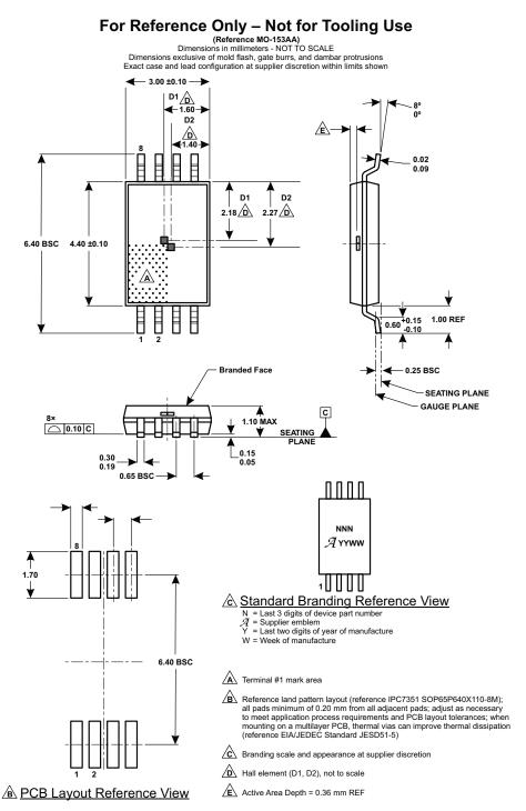
Figure 35: Package LE, 8-Pin TSSOP (Dual Die Version)
