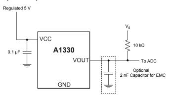
Figure 29: Typical A1330 application circuit
