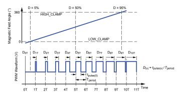
Figure 2: PWM Mode Outputs a Duty Cycle Proportional to Sensed Angle
