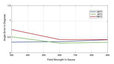
Figure 26: Typical Maximum Angle Error Over Field Strength
