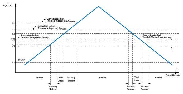
Figure 4: Relationship of V<sub>CC</sub> and Output
