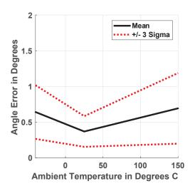
Figure 30: Peak Angle Error over Temperature (300 G)
