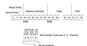
Figure 9: General Format for Serial Interface Commands
