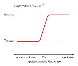
Figure 38: Effect of Saturation
