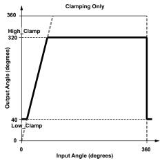
Figure 15: CE = 0, ROE = 1. Applied gain = 4×. LOW\_CLAMP = 10 (≈40°), HIGH\_CLAMP = 10 (≈320°)
