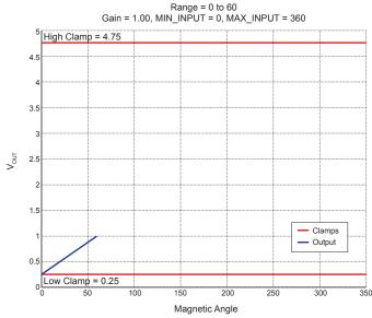
**Figure 20: Scenario C.**0-60 degree input. Gain = 1.
