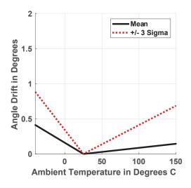
Figure 31: Maximum Absolute Drift from 25°C Reading (300 G)
