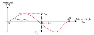
Figure 36: Angle Error Definition
