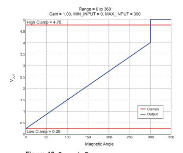
Figure 19: Scenario B. Regular 0-360 degree input value. Gain = 1. MAX\_INPUT = 300. Clamps set to 95% and 5%. Output goes into diagnostic region (in this case  $V_{CC}$ ) when input angle exceeds the MAX\_INPUT set point.
