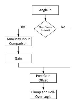
Figure 13: High Level Short Stroke Block Diagram
