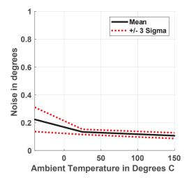
Figure 32: Noise Performance over Temperature (1 Sigma, 300 G)
