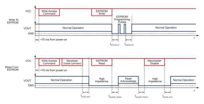
Figure 8: Programming Read and Write Timing Diagrams
