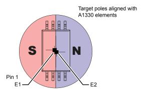
Figure 27: Orientation of Magnet Relative to Primary and Secondary Die
