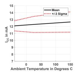
Figure 33: I<sub>CC</sub> over Temperature (V<sub>CC</sub> = 5.0 V, Analog Output)
