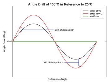
Figure 37: Angle Drift of 150°C in Reference to 25°C [1]
