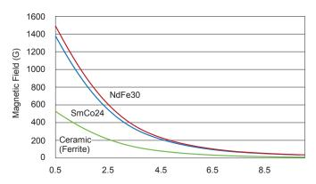
Figure 24: Magnetic Field versus Air Gap for a magnet 6 mm in diameter and 2.5 mm thick. Allegro can provide similar curves for customer application magnets upon request. Allegro recommends larger magnets for applications that require optimized accuracy performance.
