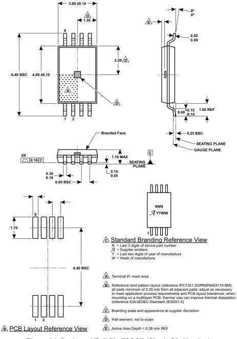
Figure 34: Package LE, 8-Pin TSSOP (Single Die Version)
