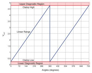
Figure 1: Output Value for a 0-720° Magnetic Input Signal
