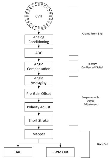
Figure 12: Digital Signal Path Description
