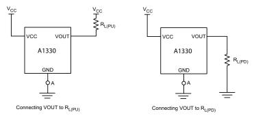
Figure 11: Connection for Detecting Broken Ground Wire
