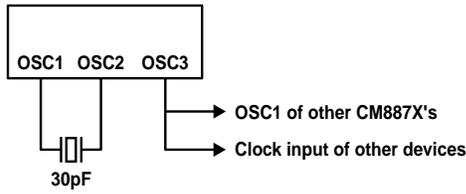
**Figure 7. CM8870C Crystal Connection (PLCC Package Only)**
