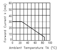
Fig.3 FORWARD CURRENT DERATING CURVE
