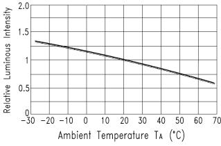
Fig.5 Luminous Intensity vs.Ambient Temperature
