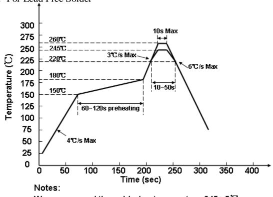
We recommend the soldering temperature 245±5℃; The maximum temperature should be limited to 260 ℃.
