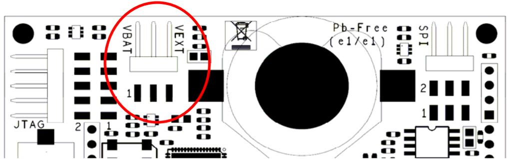
It is possible to sense whether the mega1281 runs from external supply or from battery as these voltage sources are connected to internal ADC of the mega1281. The ADC channels 0 to 4 (pins F0 to 4) are connected to various parts of the power supply network. Please refer to the schematics for more details on these connections.
