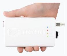
MikroProg programmer and In-Circuit Debugger supports over 570 Microchip PIC, dsPIC30/33 and PIC32 microcontrollers
