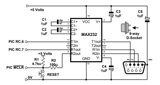
**Note:** Components R1, R2, and the Reset switch are optional, and serve to reset the microcontroller automatically. If these components are not used, the connections to R2in and R2out of the MAX232 may be omitted.
