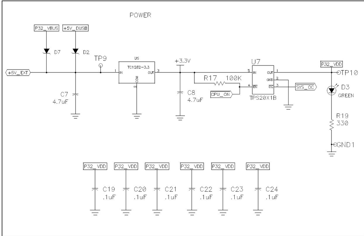
FIGURE A-8: PIC32 USB STARTER KIT II SCHEMATICS (USB OTG/DEVICE POWER SUPPLY)
