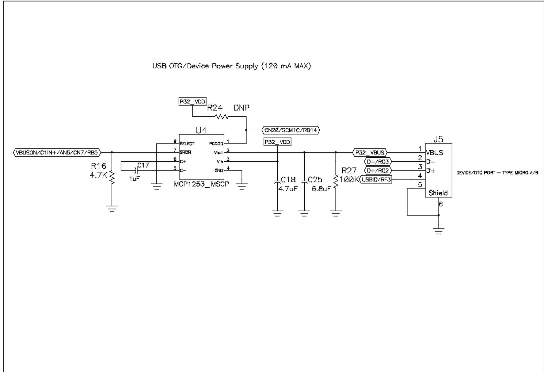
FIGURE A-9: PIC32 USB STARTER KIT II SCHEMATICS (USB HOST POWER SUPPLY)
