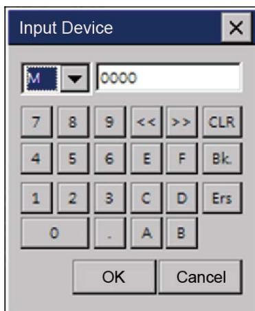
For an index device, two devices should be entered in the format of “Default Device[Index Device]”. The procedure for entering a default device is the same as the procedure for entering a general device.
