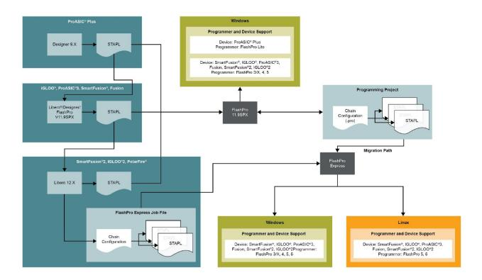
Starting with Libero SoC v12.0, The FlashPro programming software will no longer be included in the Libero design software nor will it be available in stand-alone mode. Microsemi will be supporting the FlashPro Express v12.0 programming software, which replaces the FlashPro programming software. The last versions of Libero that supports FlashPro are Libero SoC v11.9 and Libero SoC PolarFire v2.3.
