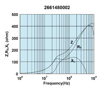
Impedance, reactance, and resistance vs. frequency.
