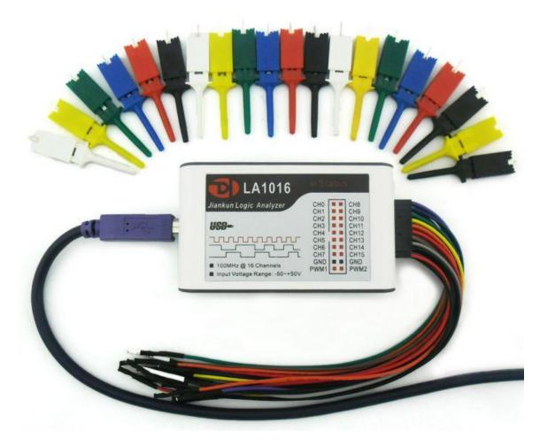
LA1016 is a high-performance logic analyzer with 16 channels and 100M sampling rate
