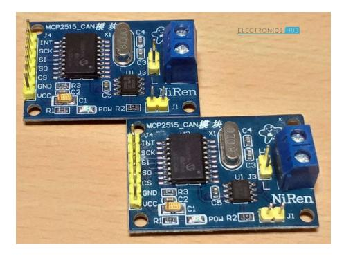
This particular module is based on MCP2515 CAN Controller IC and TJA1050 CAN Transceiver IC. The MCP2515 IC is a standalone CAN Controller and has integrated SPI Interface for communication with microcontrollers.
