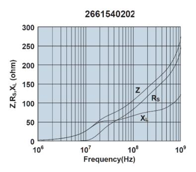
Impedance, reactance, and resistance vs. frequency.
