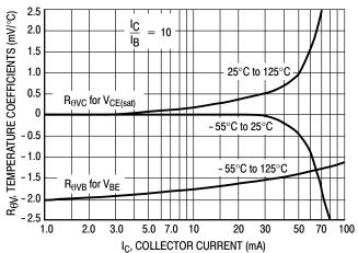
**Figure 4. Temperature Coefficients**
