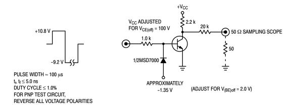
Figure 10. Switching Time Test Circuit
