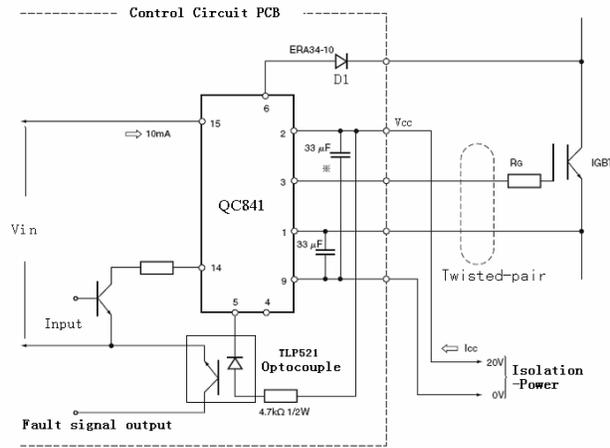
TTL compatible input interface       $f=20\text{kHz}$
