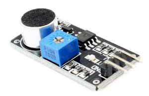
The Microphone module can be used for sound/audio detection, it comes with the basic components for you to get started. Supplying power and it is good to be use. Do take note that this sensor module can only detect the present of sound/audio, but not to differentiate the sound's level. You can use it to detect sound and further determine whether human or animal is preset in a room, maybe for light activate with clap.
