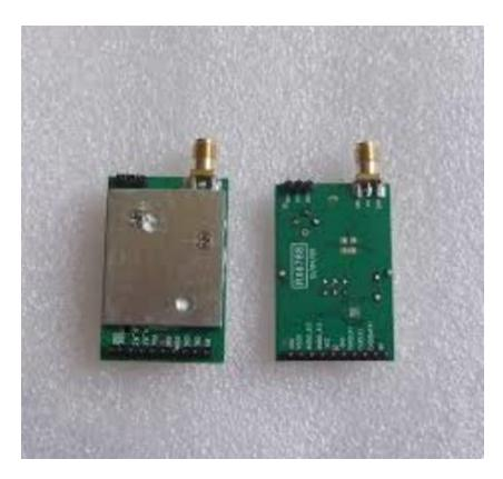
FPV 2.4GHZ 2W 16CH Wireless Audio Video Transmitter Module TX6733(2 groups of frequency, 8 channels is optional)
