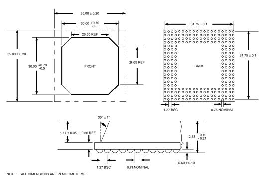
Figure 8. ISP1080/1240 352-Pin BGA Mechanical Drawings
