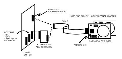
Figure 2. ATEC378 Chip Within a Host System
