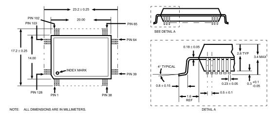
Figure 6. FAS366/366U 128-Pin PQFP Mechanical Drawings
