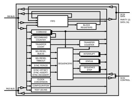
Figure 1. FAS366U Block Diagram
