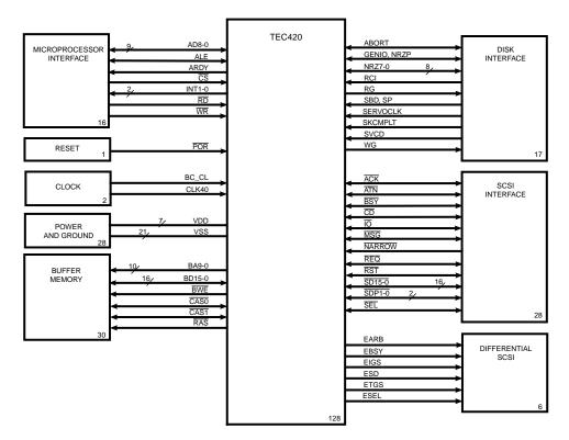
Figure 2. TEC420 Functional Signal Grouping
