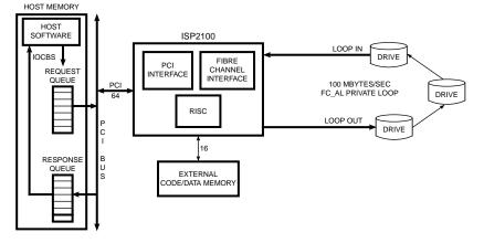
Figure 2. I/O Subsystem Design Using the ISP2100
