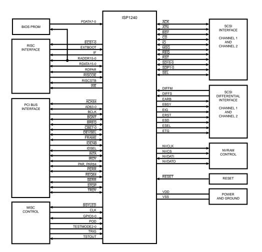
Figure 3. ISP1240 Functional Signal Grouping
