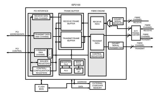
Figure 1. ISP2100 Block Diagram
