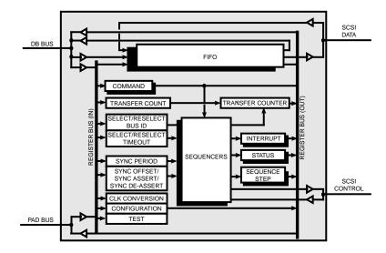
Figure 1. FAS209 Block Diagram
