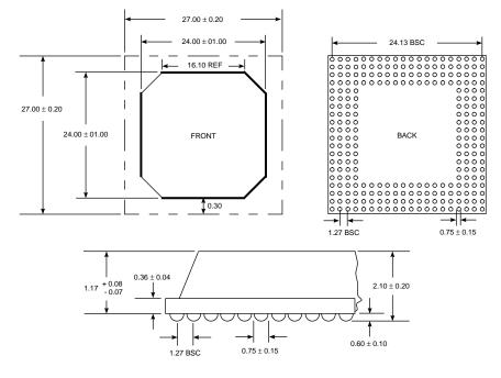
Figure 4. ISP2100 Mechanical Drawings
