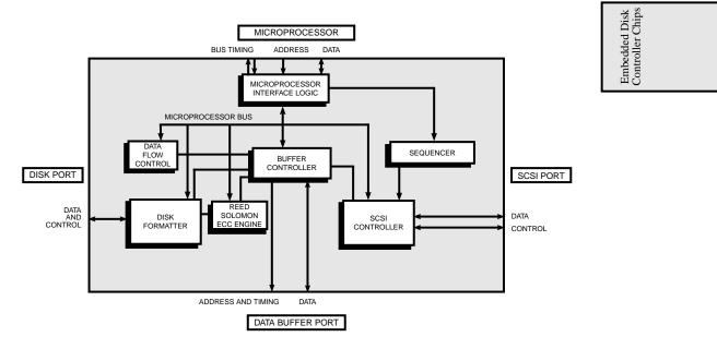
Figure 1. TEC420 Block Diagram
