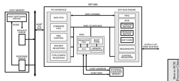
Figure 1. ISP1080 Block Diagram
