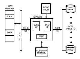
Figure 2. I/O Subsystem Design Using the ISP1000/1000U
