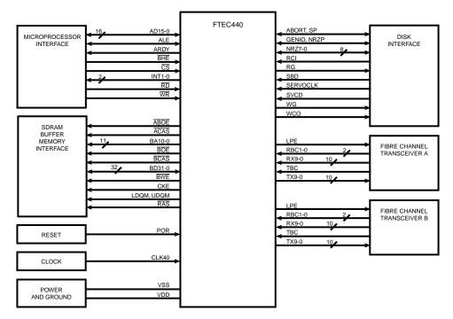
Figure 2. FTEC440 Functional Signal Grouping
