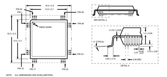
Figure 3. FAS209 64-Pin TQFP Mechanical Drawings
