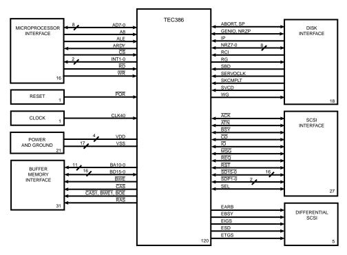
Figure 3. TEC386 Functional Signal Grouping
