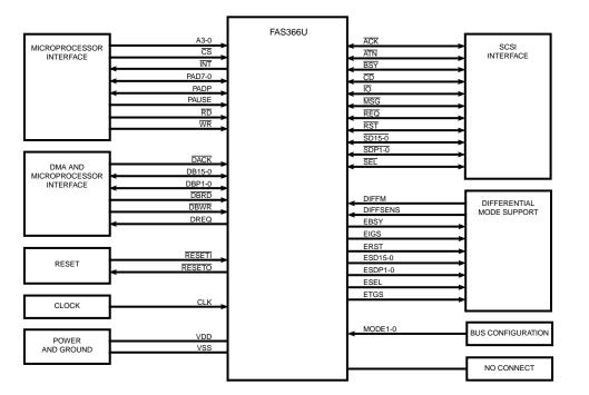
Figure 2. FAS366U Functional Signal Grouping
