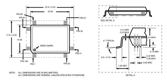
Figure 5. FAS236/236U 100-Pin PQFP Mechanical Drawings
