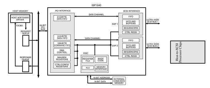
Figure 1. ISP1240 Block Diagram
