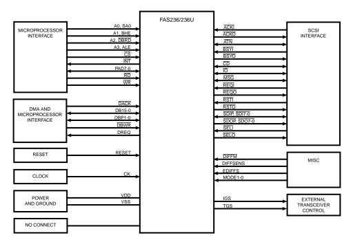
Figure 3. FAS236/236U Functional Signal Grouping
