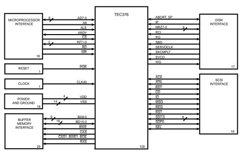
Figure 2. TEC376 Functional Signal Grouping
