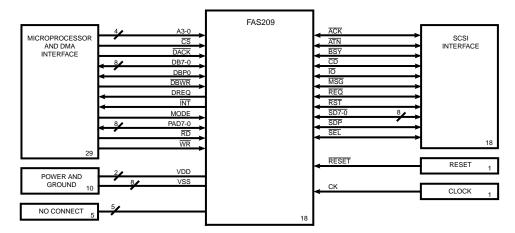
Figure 2. FAS209 Functional Signal Grouping
