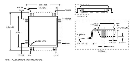
Figure 7. ISP1000/1000U/1040B 208-Pin PQFP Mechanical Drawings
