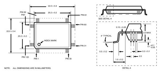
Figure 12. TEC386 120-Pin PQFP Mechanical Drawings
