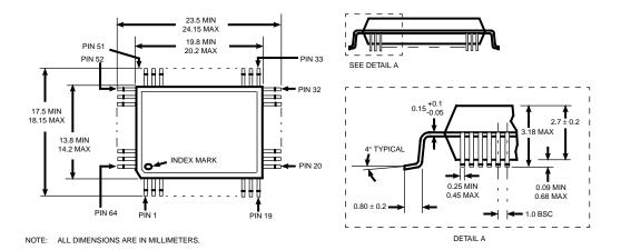
Figure 2. FAS209 64-Pin PQFP Mechanical Drawings
