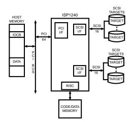
Figure 2. I/O Subsystem Design Using the ISP1240
