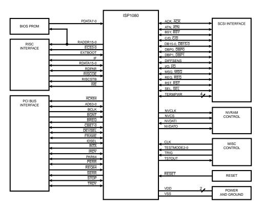
Figure 3. ISP1080 Functional Signal Grouping
