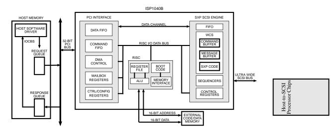
Figure 1. ISP1040B Block Diagram
