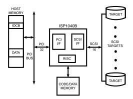
Figure 2. I/O Subsystem Design Using the ISP1040B
