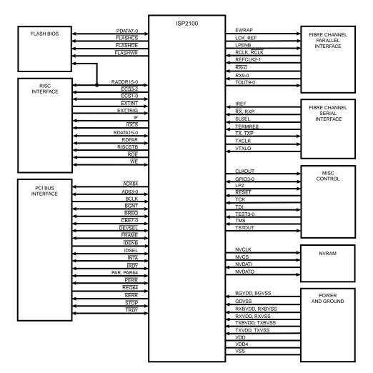
Figure 3. ISP2100 Functional Signal Grouping
