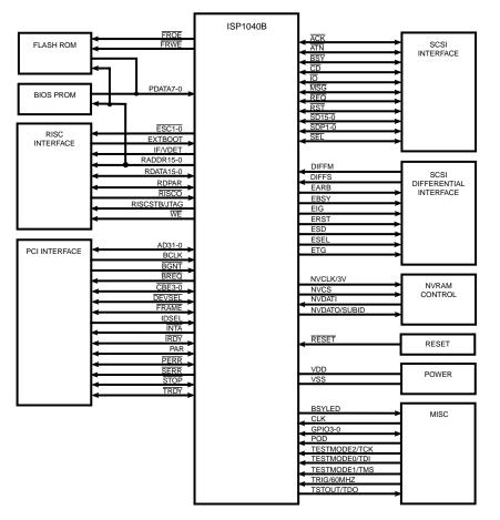
Figure 3. ISP1040B Functional Signal Grouping
