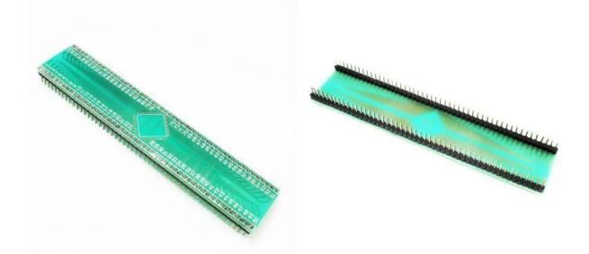
TQFP-100 to DIP-100 SMT Adapter (0.4 mm pitch, 12 x 12 mm body)
