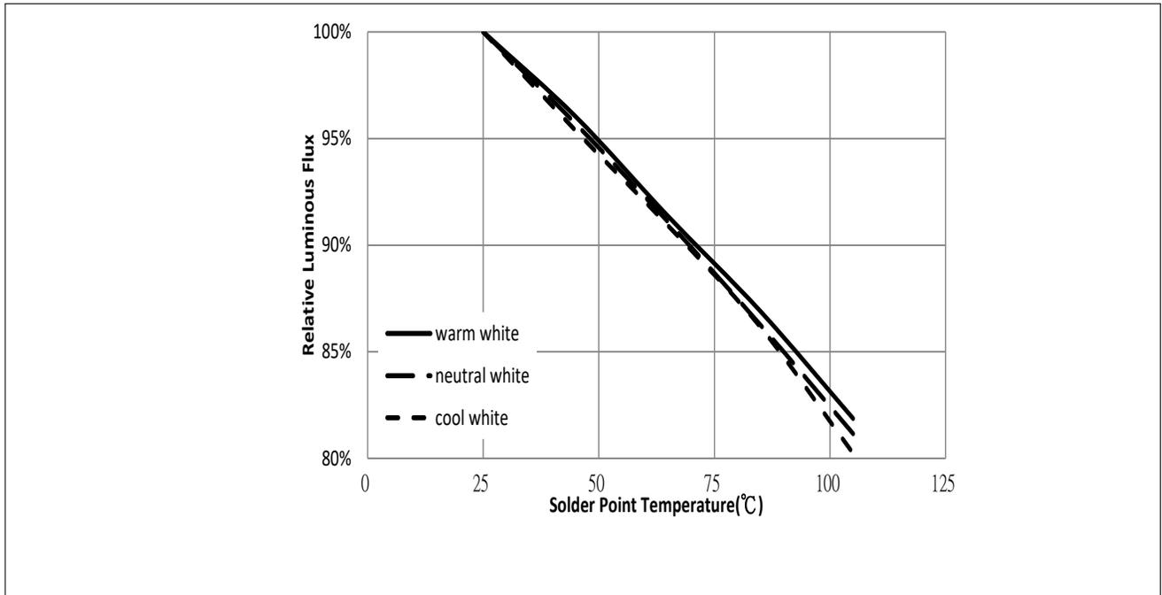
**Figure 5: Typical cxx Shift vs. Solder Point Temperature**
