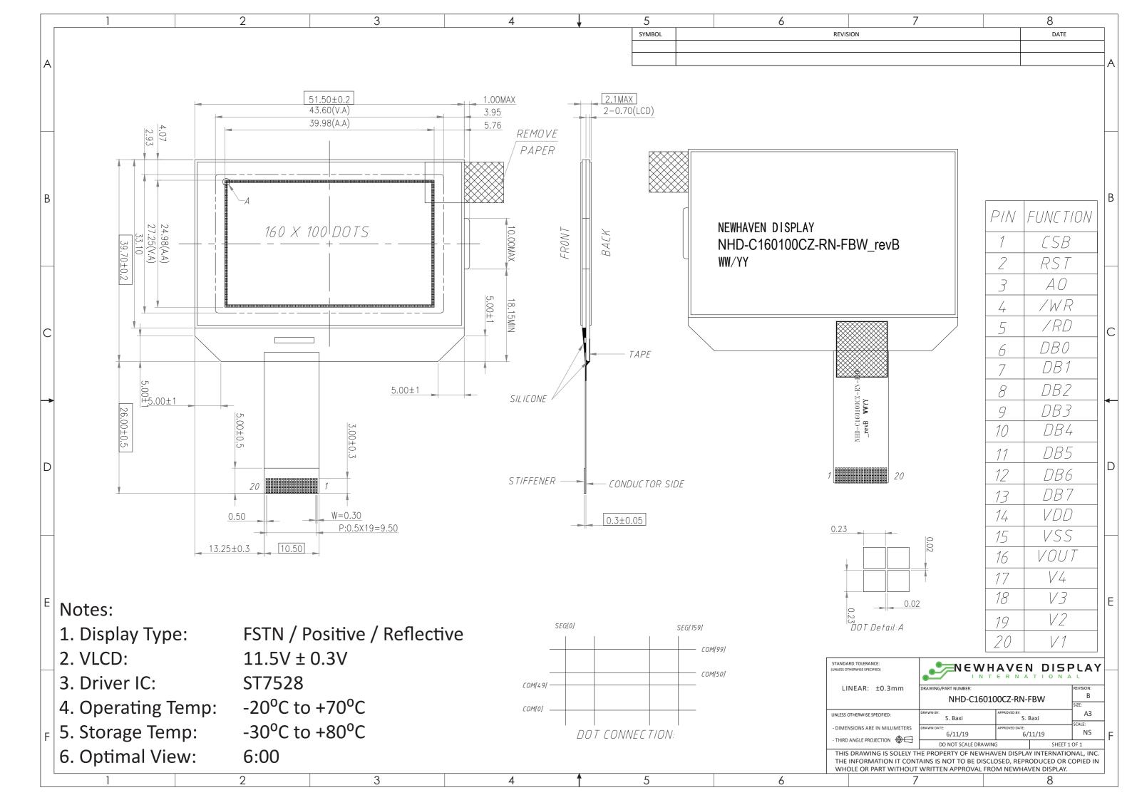
**Pin Description and Wiring Diagram**
