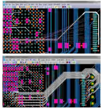
New routing technology allows the designer to sketch the path of signals, then the interactive router efficiently routes those traces. In the top image, the designer has "sketched" the path desired for the signals shown in purple. In the bottom illustration, the Sketch Router has efficiently routed the traces according to the designer's sketch.
