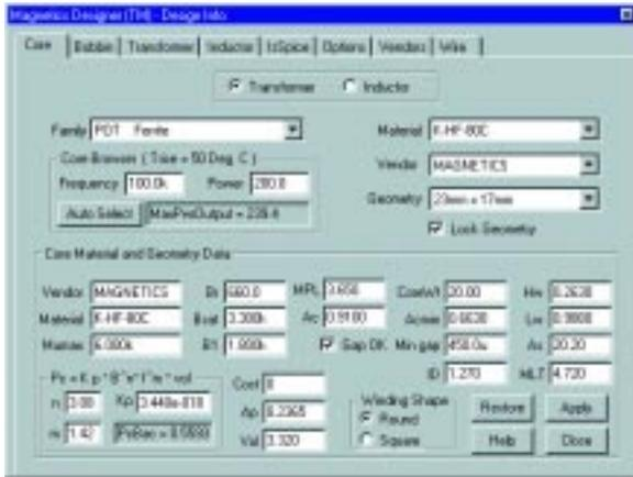
The **Core Selection Screen** (above) gives you thousands of cores to choose from. The database is extensible, allowing you to add your own “exotic” cores, materials, and wire information. A database of core manufacturers, core distributors, wire distributors, and transformer manufacturers is also included, along with the ability for you to add your favorite vendor to the list.
