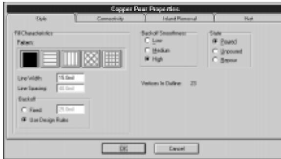
Finally click the radio button marked **Poured** and the **OK** button, then watch ACCEL EDA work.
