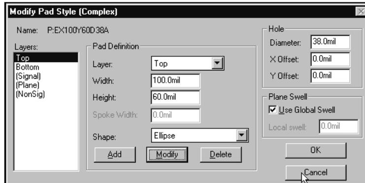
Exit the dialog without making changes. Switch your current layer to the Top, Bottom, and a middle signal layer, choosing View Redraw after each layer change. Notice the shape and size of the pads on each layer matches the stackup definition.
