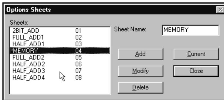
In particular notice the two full adder sheets and four half adder sheets (two for each full adder). Looking at these closer, you’ll see reference designators have been uniquely assigned to the components.
