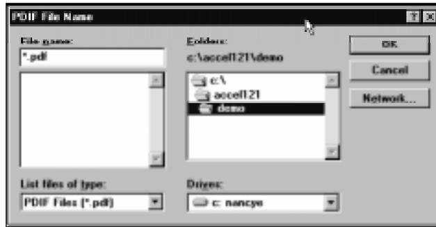
2. Select the type of file to load. You can either select PDFIF Files if you want to load a .PDF file, or select .CFG Files if you want to load a design.cfg file for a particular schematic. We recommend that you load the design.cfg file if your schematic design is a multi-sheet design.
