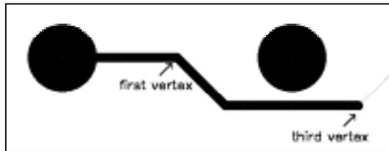
6. When the mouse is down, press the *O* key to access the desired orthogonal shape and the *F* key to toggle the vertex. Release the mouse. Notice the second vertex is added for you. The orthogonal modes include arcs, 45 degree diagonals, and 90 degree angles.
