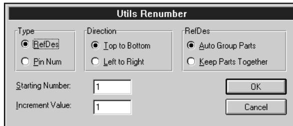
Leave the dialog settings as they are and click **OK**. Your reference designators will be renumbered in top-to-bottom order within prefix types. In particular, your resistors are renumbered starting with R1, and the IC's are renumbered starting with U1. Notice also, renumbering of U3 and U4 was done across sheets.
