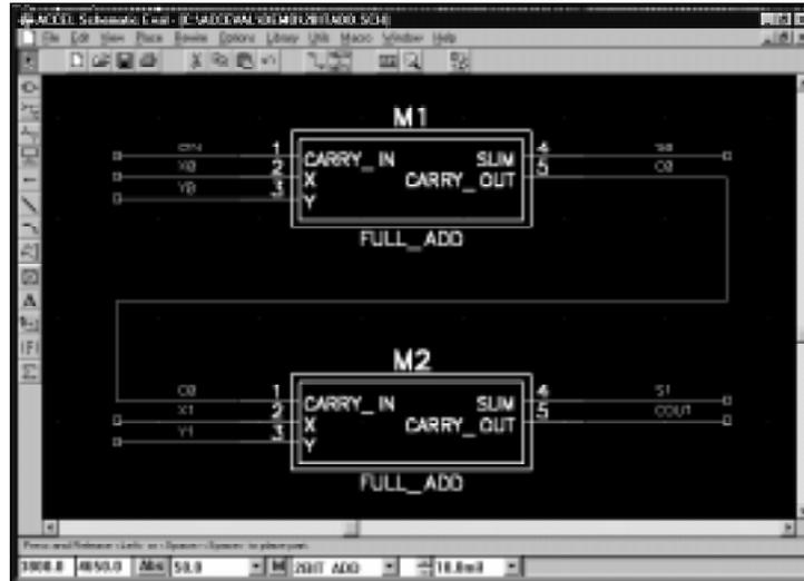
Examine component M1 or M2 on sheet 2BIT\_ADD. The M reference designator prefix indicates it is a module; a *black box* component that abstractly represents a sub-circuit. It has three input pins and two output pins, each representing an input or output of the sub-circuit.
