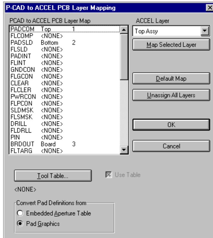
5. At the P-CAD to ACCEL PCB Layer Mapping dialog box, select the appropriate layer mapping assignments. For details about mapping layers, see the section “Mapping Layers from P-CAD Binary and PDIF Files to PCB.”
