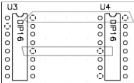
Create a second rectangle around the pads of net A3 (the net connecting pad 12 of U3 with pad 5 of U4). Again modify the split, this time setting the **Net** to A3. Any number of splits can be similarly created and assigned. For clearer viewing, the extra connection lines have been hidden in the following picture.
