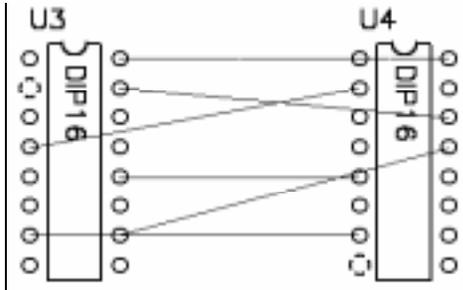
With the plane layer still active, select the Split Plane tool and create a polygon around the pads of net A1 (upper connection line) adding a new grid if necessary (see upper polygon in the diagram below). Modify the split (activate the Select tool and double-click in the area) to set the **Net** to A1 and change the **Net Plane Color**. Notice the pads in A1 are automatically tied to the split.
