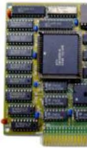
ATI "Graphics Solution Rev 3" from 1985/1986, supporting [Hercules](#) graphics. As the [PCB](#) reveals, the layout dates from 1985, whereas the marking on the central chip *CW16800-A* says "8639" - meaning that chip was manufactured in week 39, 1986. Notice [UM6845E CRT controller](#). This card uses the [ISA 8-bit interface](#).
