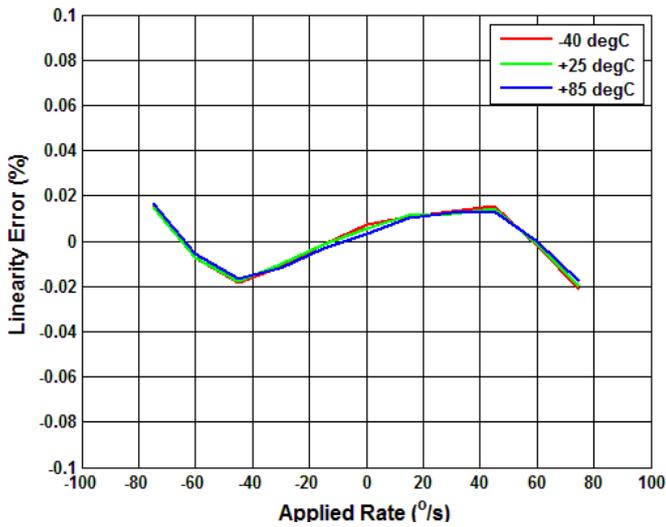
Figure 5.33 Digital Ave Error (%) vs Applied Rate
