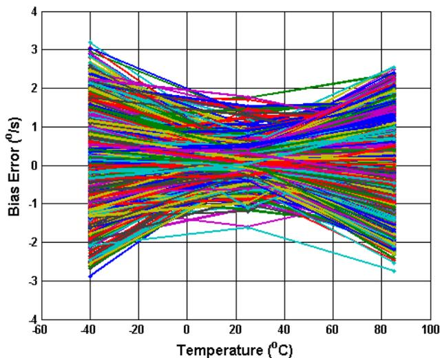
**Figure 5.2 Analogue Bias Error (dsp) vs Temperature**
