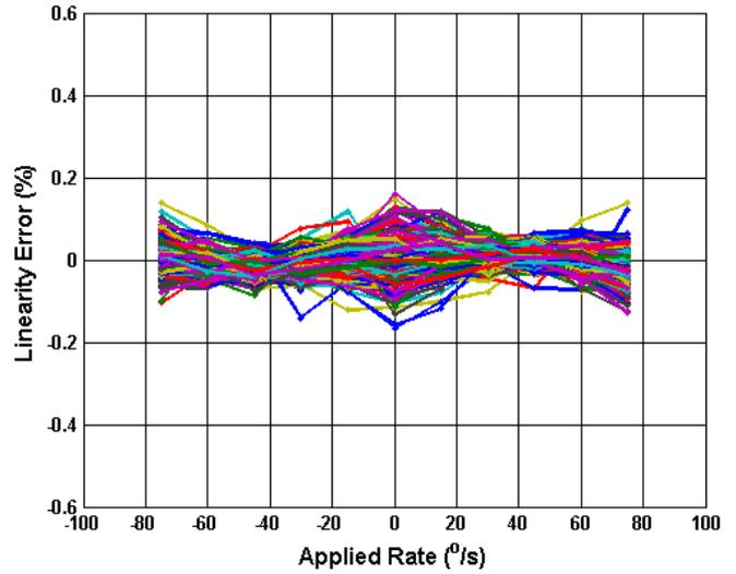
**Figure 5.31 Digital NL Error (%) vs Applied Rate (25°C)**
