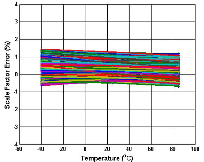
**Figure 5.28 Digital Scale Factor Error (%) vs Temperature**
