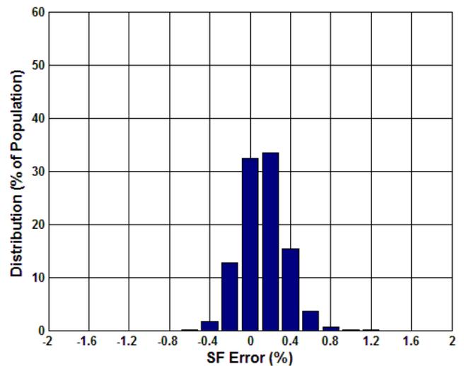
Figure 5.40 Digital SF Error (%) at 25°C
