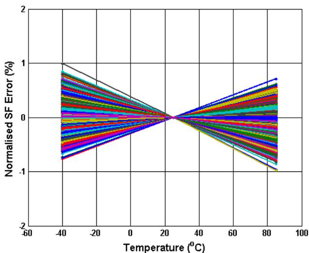
**Figure 5.6 Analogue Normalised Scale Factor Error (%) vs Temperature**
