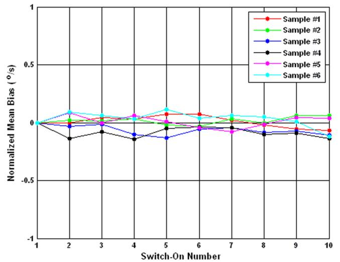
Figure 5.51 Switch-On Repeatability of Normalised Mean Bias
