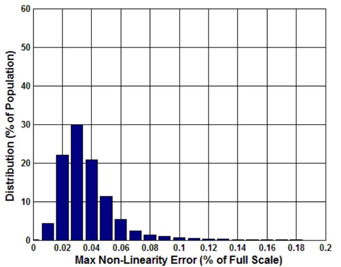
**Figure 5.44 Digital Maximum Linear Error (%) at 85°C**
