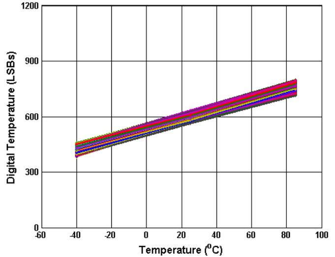
**Figure 5.27 Digital Temperature Output (LSB) vs Temperature**
