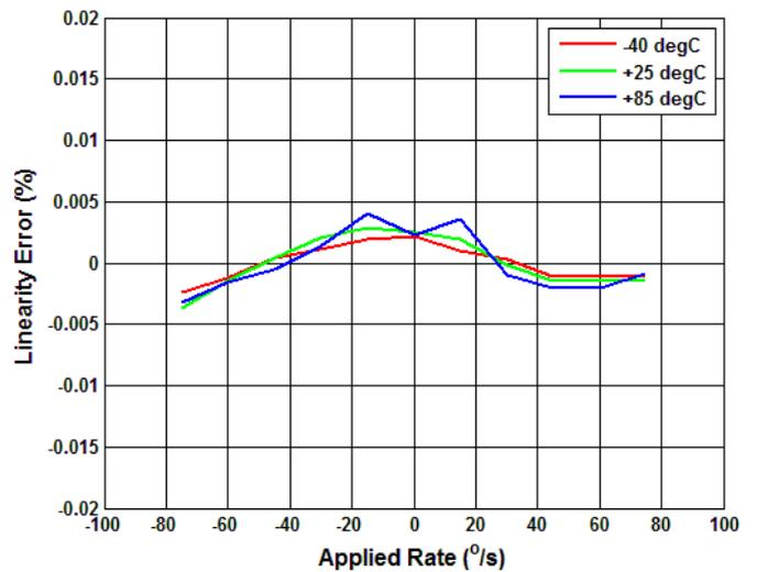
**Figure 5.7 Analogue Ave NL Error (%) vs Applied Rate**
