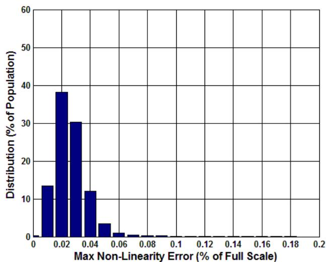
**Figure 5.22 Analogue Maximum Linear Error (%) at -40°C**
