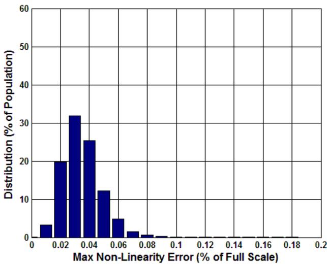
**Figure 5.42 Digital Maximum Linear Error (%) at -40°C**
