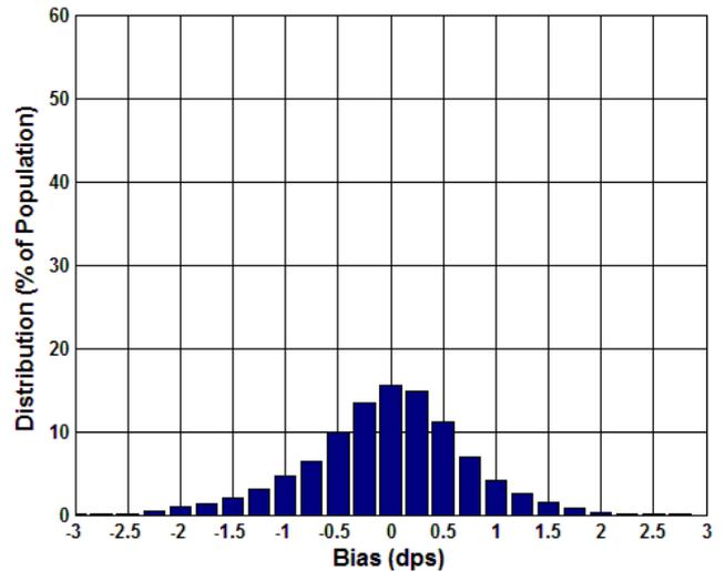
Figure 5.15 Analogue Normalised Bias Distribution (dps) Over Temperature
