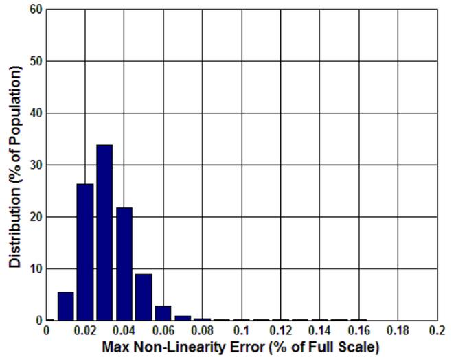
**Figure 5.43 Digital Maximum Linear Error (%) at 25°C**
