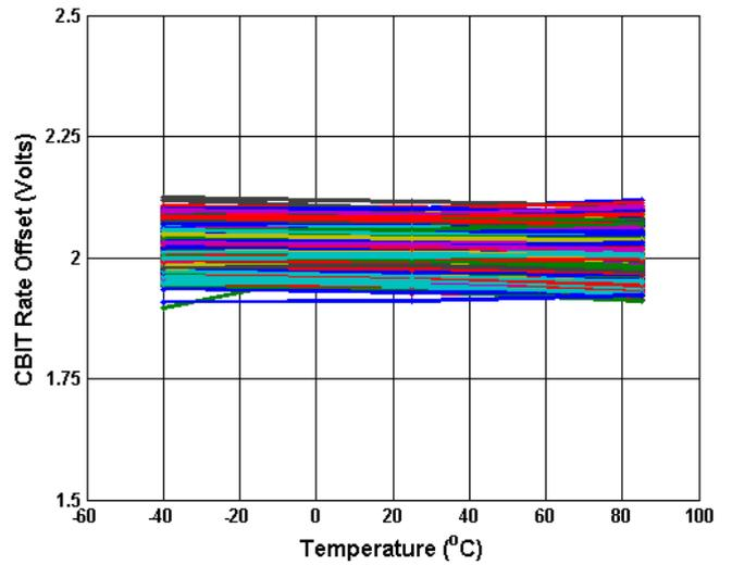
**Figure 5.11 Analogue CBIT Offset (Volts) vs Temperature**
