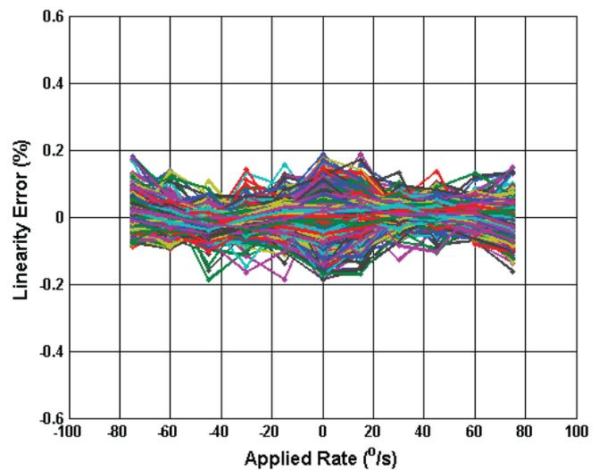
**Figure 5.32 Digital NL Error (%) vs Applied Rate (85°C)**
