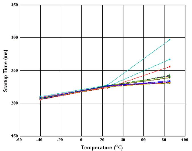
Figure 5.48 Startup Time vs Temperature (Vdd = 2.7V)
