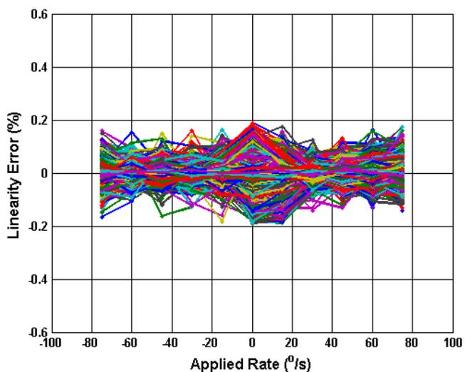
**Figure 5.10 Analogue NL Error (%) vs Applied Rate (85°C)**
