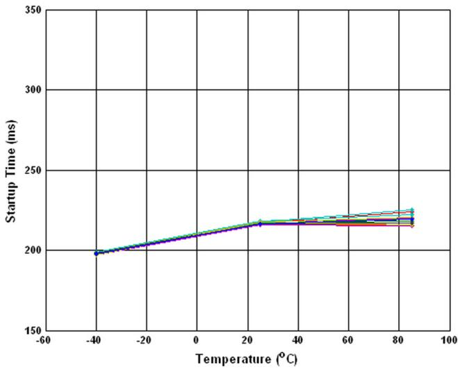
Figure 5.49 Startup Time vs Temperature (Vdd = 3.6V)
