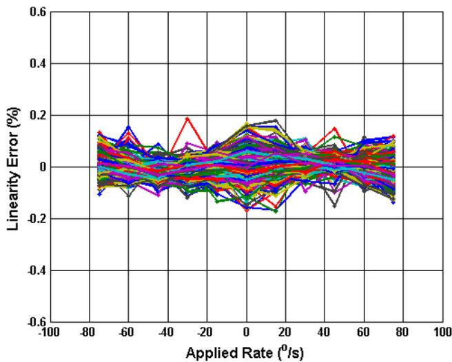
**Figure 5.30 Digital NL Error (%) vs Applied Rate (-40°C)**
