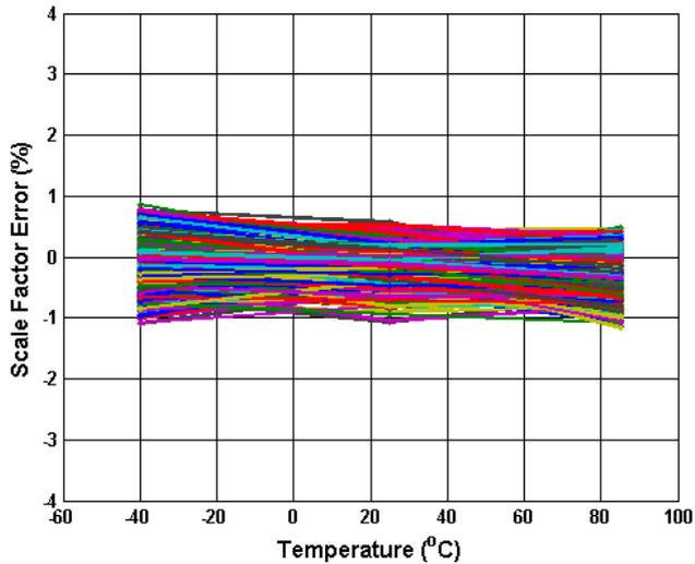
**Figure 5.5 Analogue Scale Factor Error (%) vs Temperature**
