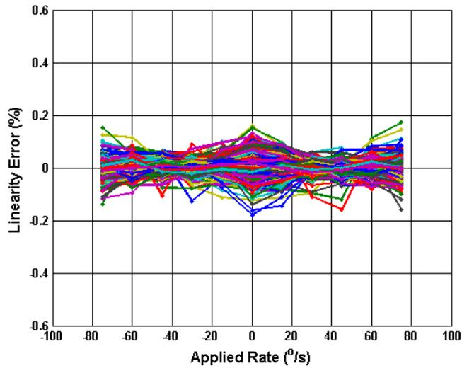
**Figure 5.9 Analogue NL Error (%) vs Applied Rate (25°C)**
