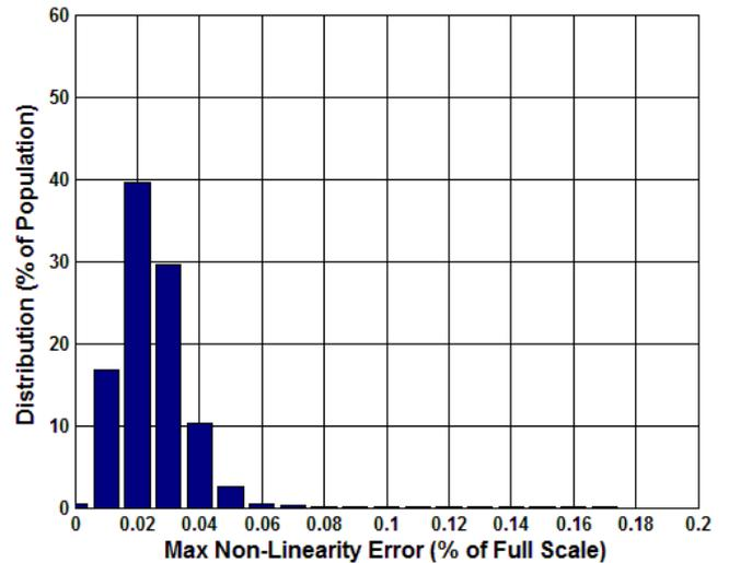
**Figure 5.23 Analogue Maximum Linear Error (%) at 25°C**
