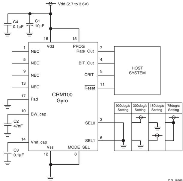
**Figure 7.3 Peripheral Circuit - Analogue Output (CRM100)**
