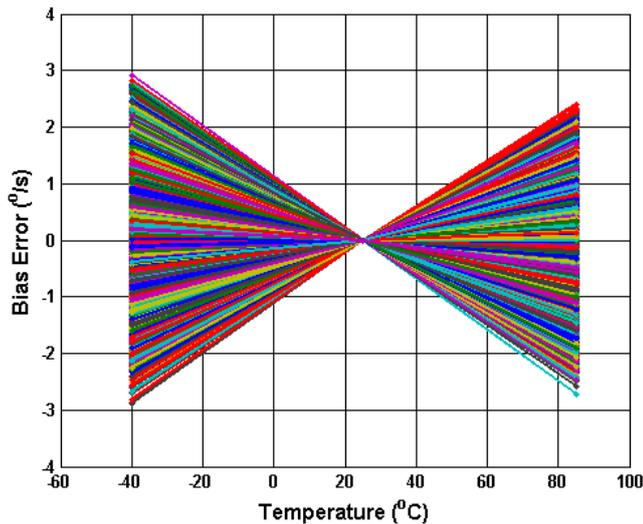
**Figure 5.26 Digital Normalised Bias Error (dps) vs Temperature**
