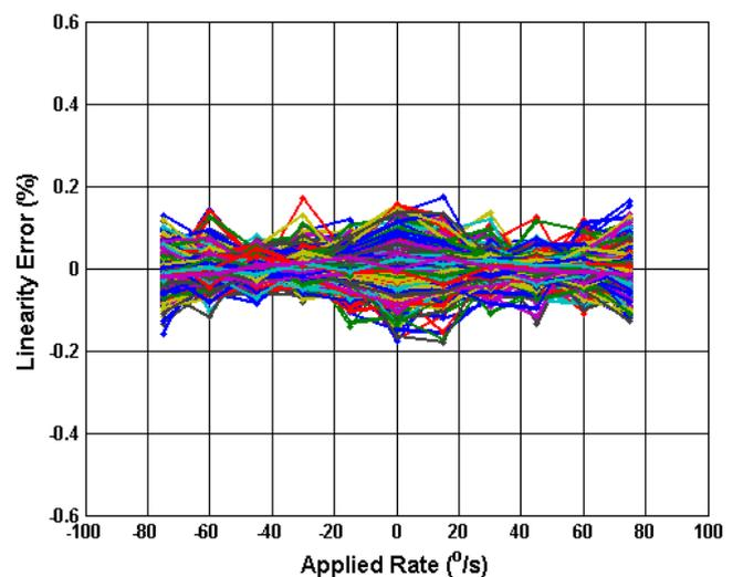
**Figure 5.8 Analogue NL Error (%) vs Applied Rate (-40°C)**
