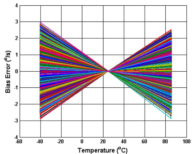
**Figure 5.3 Analogue Normalised Bias Error (dps) vs Temperature**
