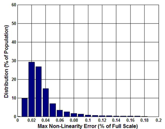
**Figure 5.24 Analogue Maximum Linear Error (%) at 85°C**
