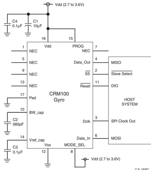
**Figure 7.4 Peripheral Circuit - Digital Output (CRM100)**
