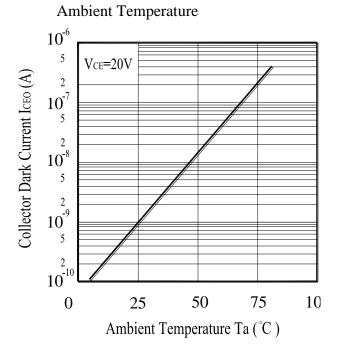
Fig.6 Collector Current vs.
