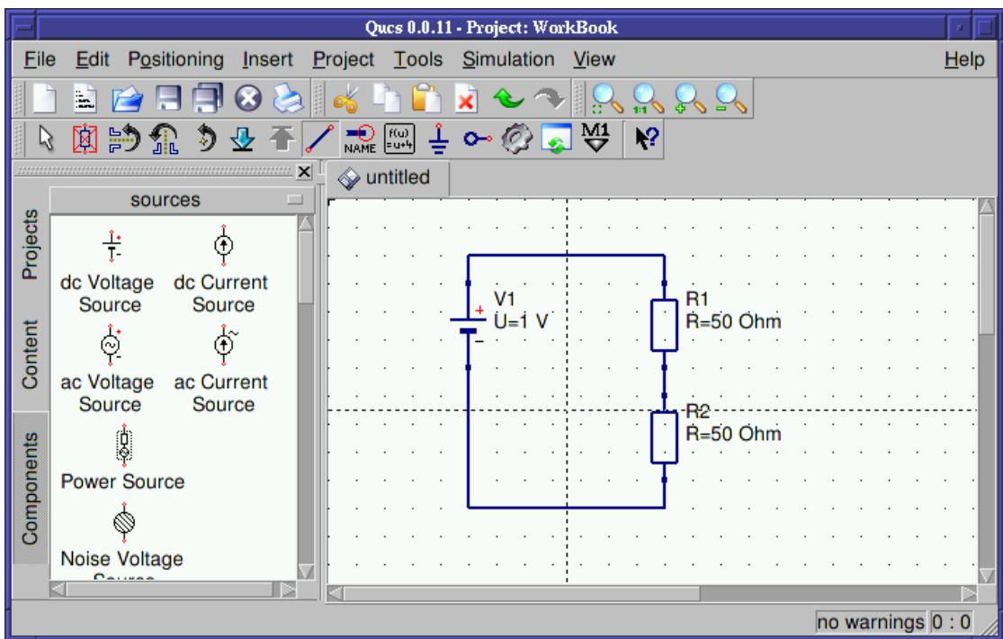
Figure 7: Components of the voltage divider appropriately wired
