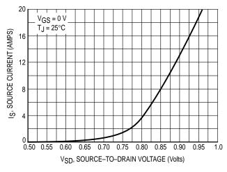
Figure 10. Diode Forward Voltage versus Current
