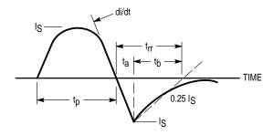
Figure 15. Diode Reverse Recovery Waveform
