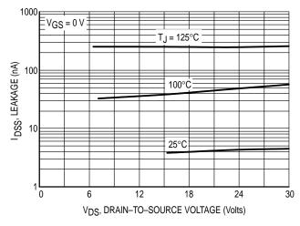
Figure 6. Drain–To–Source Leakage Current versus Voltage
