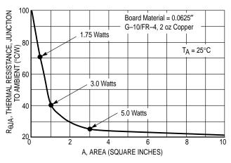
Figure 16. Thermal Resistance versus Drain Pad Area for the DPAK Package (Typical)
