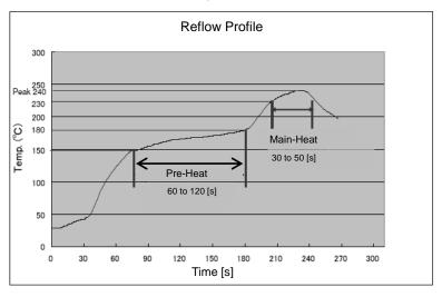
fig.1 Example of recommended temperature profile for reflows
