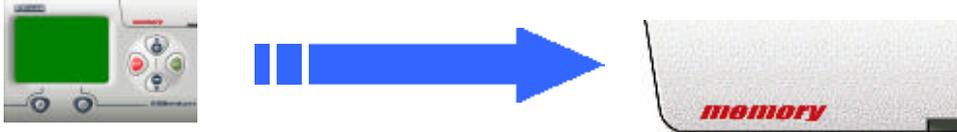
Insert the memory module into the Millenium with the front panel unlocked. Saves are performed in stop mode.
