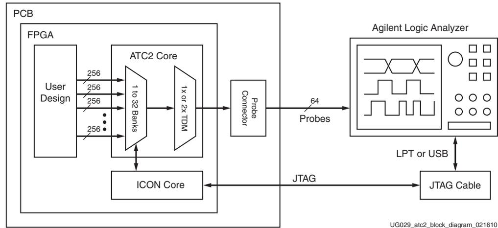
Figure 1-4: ATC2 Core and System Block Diagram
