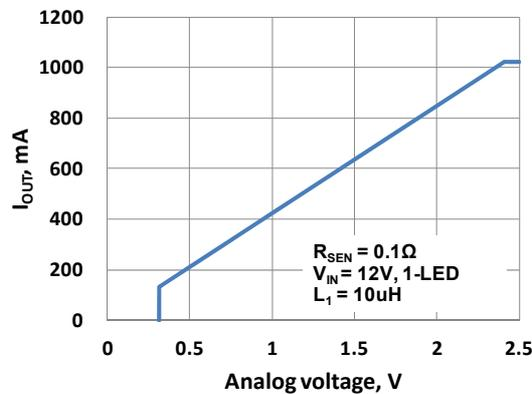
Fig. 16 Analog dimming curve
