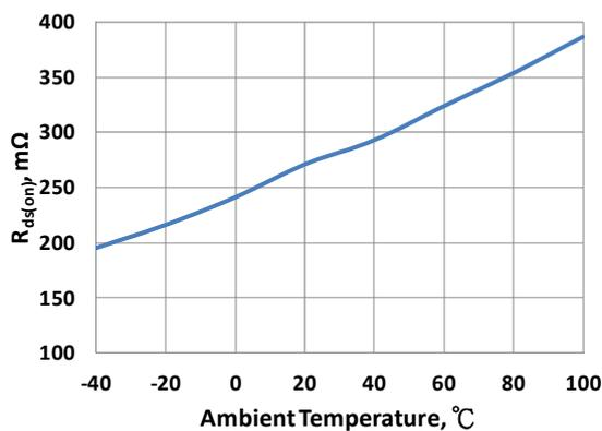
Fig. 13  $R_{ds(on)}$  vs. Ambient Temperature at  $V_{IN} = 12V$
