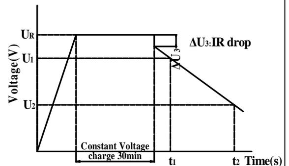
Figure2. Curve for charge-discharge
