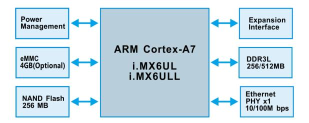
Figure 1-3 MYC-Y6ULX-V2 Function Block Diagram
