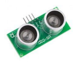
The US-020 ultrasonic sensor uses sonar to determine distance to an object like bats or dolphins do. It offers excellent range accuracy and stable readings in an easy-to-use package. It operation is not affected by sunlight or black material like infrared rangefinders are (although acoustically soft materials like cloth can be difficult to detect).
