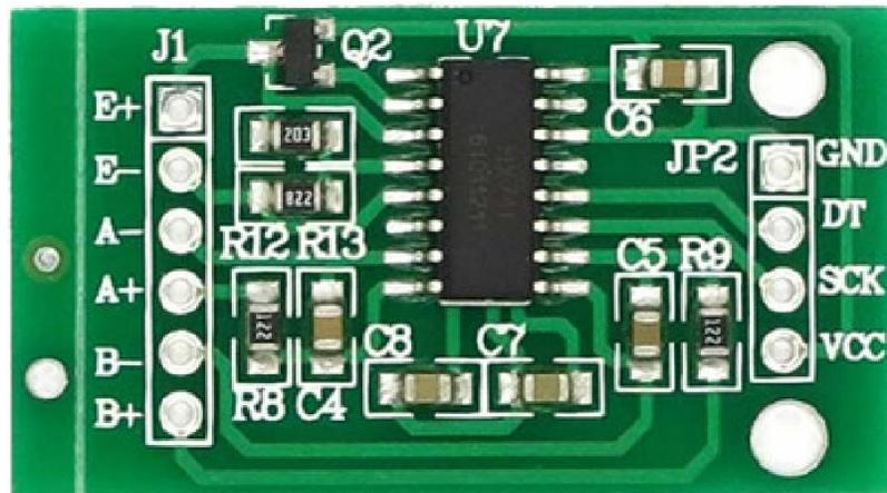
Simply connect Load cell wires to the HX711 module based on their color, then connect DAT (Data) pin to Arduino Analog pin A1 and connect CLK (Clock) pin to Arduino Analog pin A0, Put Vcc and Gnd supply from Arduino power source pins.
