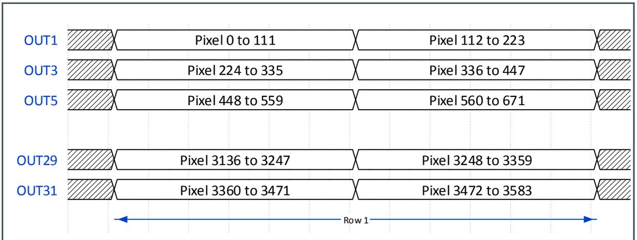
In 8-channel mode, one row is read out over 8 data channels in four bursts of 112 pixels.
