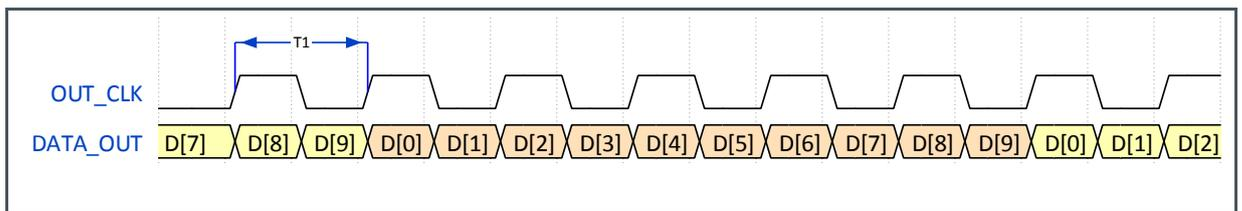
For 10-bit mode, the time 'T1' in Figure 26 will be equal to 1 clock cycle of the IN\_LCLK input clock. When a frequency of 300 MHz (max for 10-bit mode) is applied to IN\_LCLK, this results in a 300 MHz OUT\_CLK.
