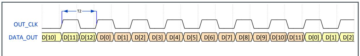
For 12-bit mode, the time 'T2' in the above figure will be equal to 1 clock cycle of the IN\_LCLK input clock. When a frequency of 300 MHz is used for IN\_LCLK (maximum in 12-bit mode), this results in a 300 MHz OUT\_CLK.
