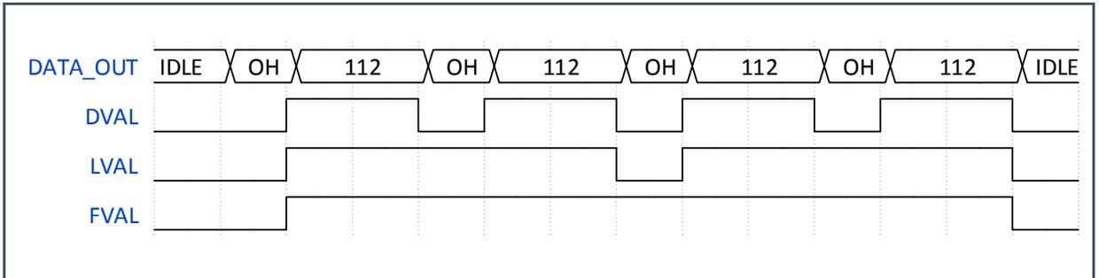
When only 8-channels are used, the line read-out time is 2 times longer. The control channel considers this and adjusts the sync codes (LVAL) to suit the slower read-out. The timing extrapolates identically for 4 and 2 channel read-out.
