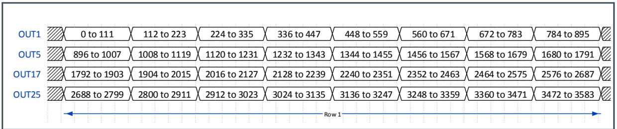
In 2-channel mode, one row is read out over 2 data channels in sixteen bursts of 112 pixels.
