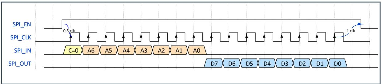
For reading several register sequentially, the SPI\_EN signal stays at a high level in the same fashion as with the write command.
