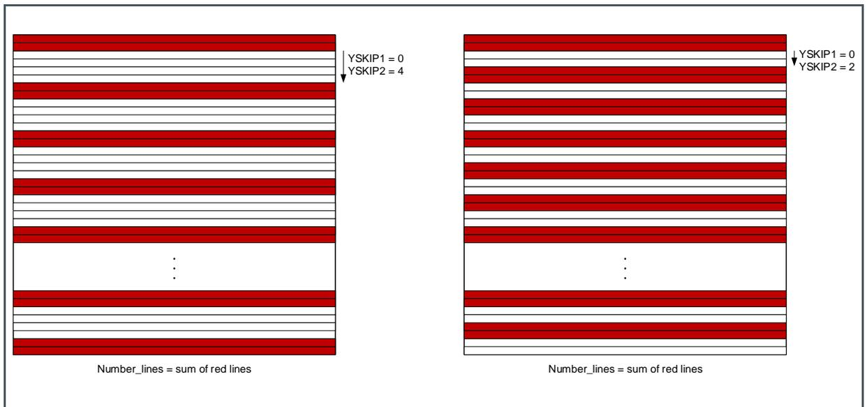
For a monochrome sensor, the values of YSKIP1 and YSKIP2 should be equal to skip single or multiple lines.
