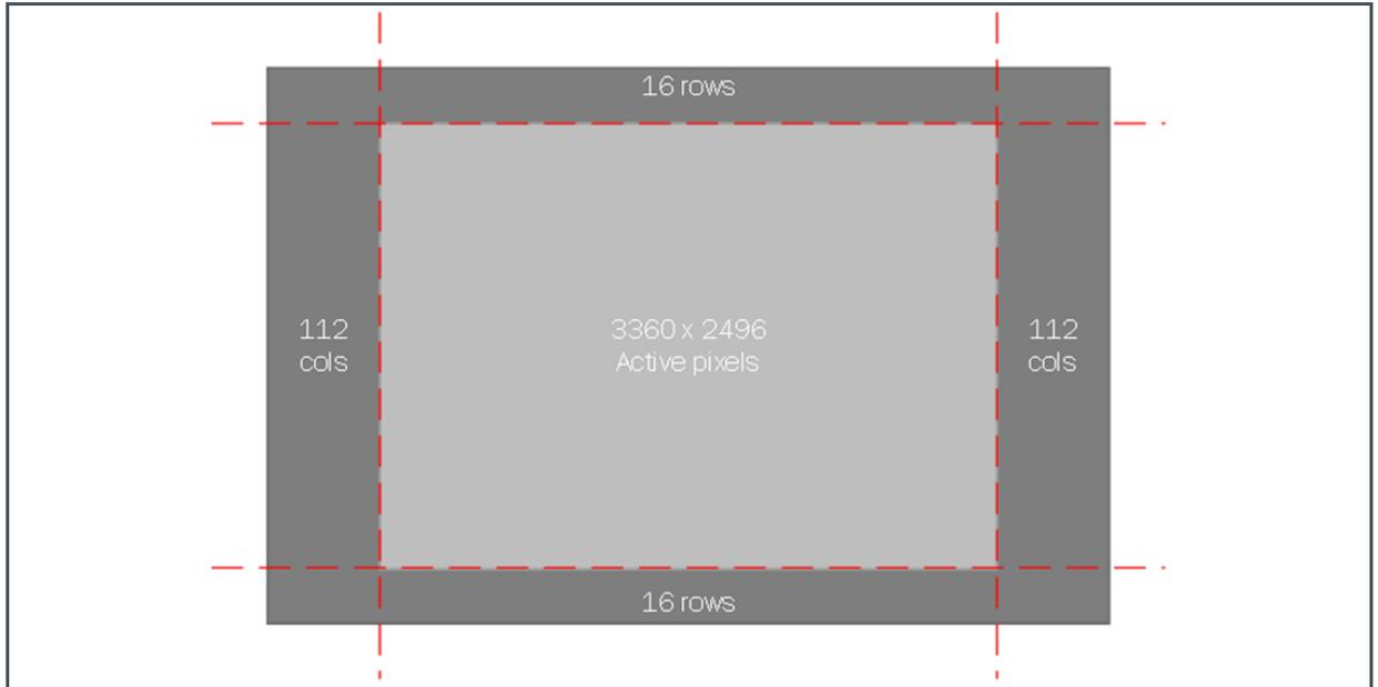
To ensure that the electrical black rows are always read out first by the sequencer, these rows are assigned the 32 lowest logical addresses. When the image is mirrored in the Y-direction, the black rows will still be read out first, from row31 to row0, followed by the active pixels on row32 to row2527. In the image below, the pixel array is plotted to the logical addresses, instead of the physical location.
