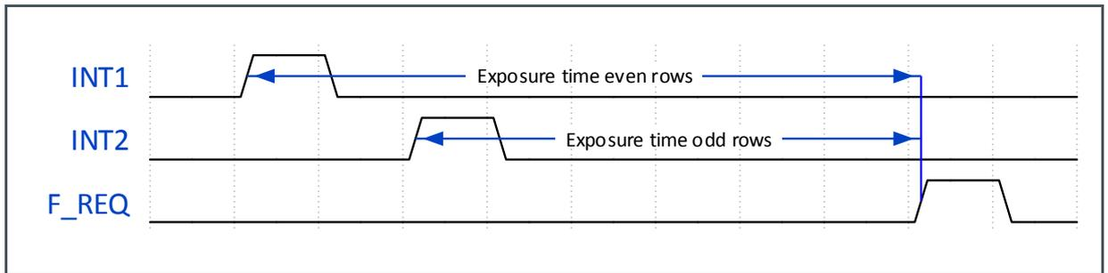
When a color sensor is used, the dual exposure mode has to be adjusted to preserve the Bayer pattern. By enabling the following register, the two exposure groups are valid for two adjacent columns.
