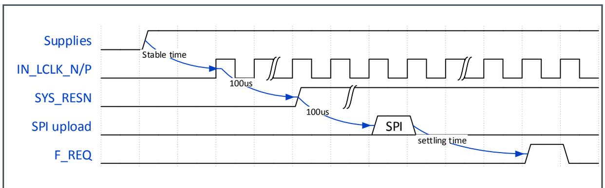
If a sensor reset is necessary during sensor operation, the same sequence should be followed, starting from the rising edge on the SYSRESN pin. A reset action (falling edge on SYSRESN) triggers all programmable registers to return to their default value. After a reset sequence, a minimum time of 1  $\mu$ s needs to be respected before a frame is requested with the F\_REQ pin.
