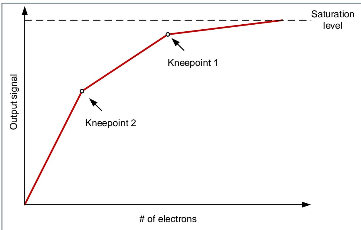
This mode can be both used in internal and external exposure mode. In the latter case, only the VTGLOW registers need to be set and the kneepoints are controlled by pulsing the INT1 signal, as shown in Figure 43.
