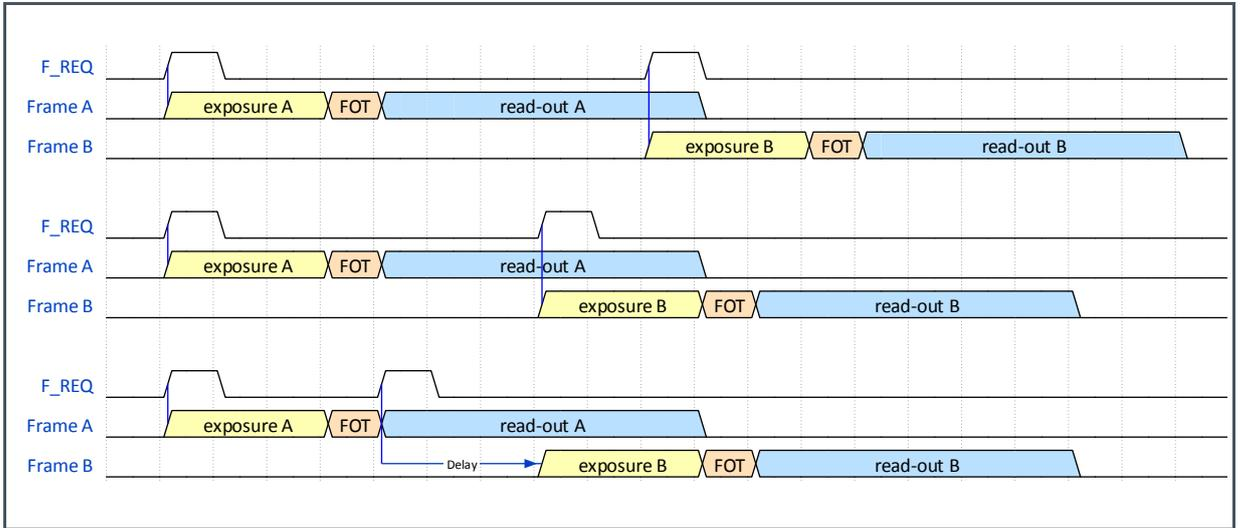
In some cases the F\_REQ timing is such that the exposure start of FRAME B would trigger the read-out period of FRAME B to start when the read-out period of FRAME A has not yet finished, causing a timing conflict.
