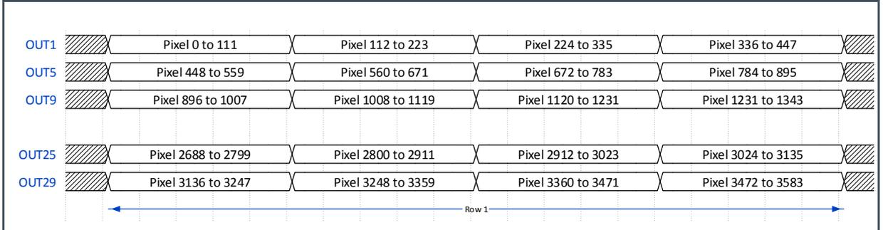
In 4-channel mode, one row is read out over 4 data channels in eight bursts of 112 pixels.
