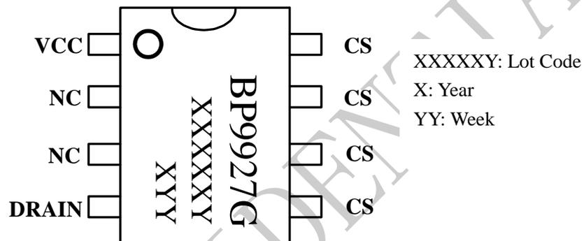
Figure 2. Pin configuration
