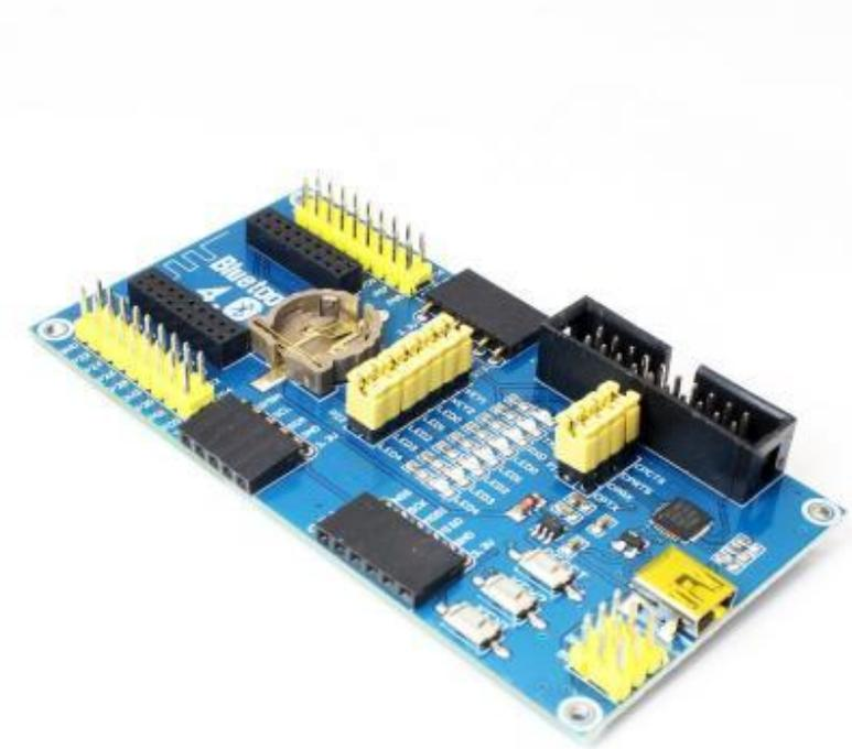
ble4.0 development board Bluetooth module nRF51822 backplane needs to be equipped with nRF51822 core board
