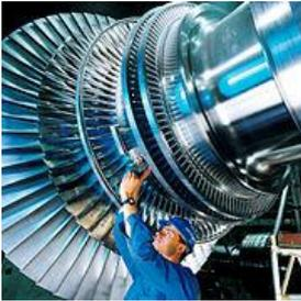
A Siemens steam turbine rotor
