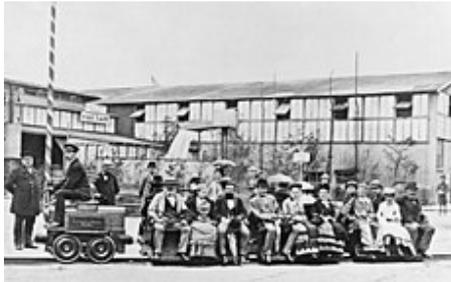
First [electric locomotive](#), built in 1879 by company founder Werner von Siemens.
