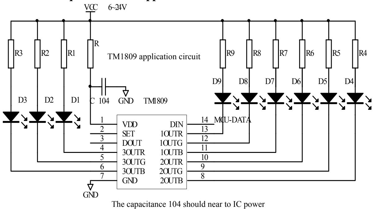
According to different supply power voltage, different resistance is requested to add between power supply interface and VDD PIN of TM1809. The resistance as the below for application reference,
