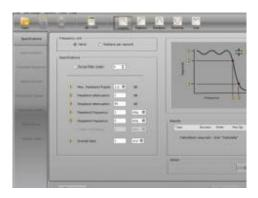
Active filter design software for lowpass, highpass, bandpass and bandstop electronic filters using resistors, capacitors and op amps. Provides Butterworth, Chebyshev, Elliptic and Bessel Approximations to order 20, with a variety of circuit choices.
