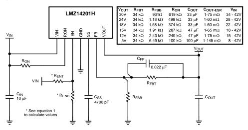
Figure 46. Simplified Application Schematic
