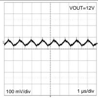
Figure 34. Output Ripple  $V_{IN}$  = 24 V,  $I_{OUT}$  = 1 A, Polymer Electrolytic  $C_{OUT}$ , BW = 200 MHz
