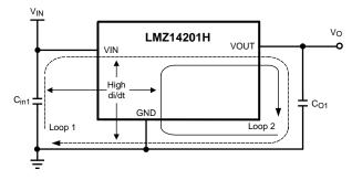
Figure 49. Critical Current Loops to Minimize
