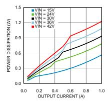
Figure 51. Power Dissipation  $V_{OUT} = 12 \text{ V}, T_A = 85^{\circ}\text{C}$
