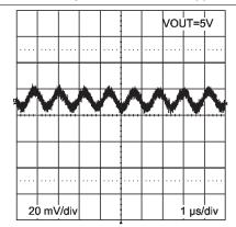
$\label{eq:Vin} Figure~33.~Output~Ripple \\ V_{IN} = 12~V,~I_{OUT} = 1~A,~Ceramic~C_{OUT},~BW = 200~MHz$
