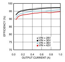
Figure 47. Efficiency  $V_{OUT} = 24 \text{ V}$ ,  $T_A = 25^{\circ}\text{C}$
