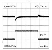
Figure 36. Load Transient Response  $V_{IN}$  = 24 V  $V_{OUT}$  = 12 V Load Step From 30% to 100%
