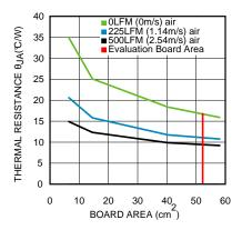
Figure 52. Package Thermal Resistance R<sub>0JA</sub> 4-Layer PCB With 1-oz Copper
