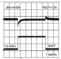
Figure 35. Load Transient Response  $V_{\rm IN}$  = 24 V  $V_{\rm OUT}$  = 12 V Load Step from 10% to 100%
