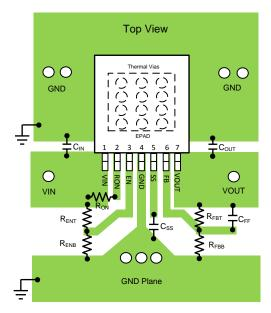
Figure 50. PCB Layout Guide
