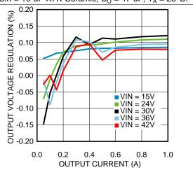
Figure 32. Line and Load Regulation T<sub>A</sub> = 25°C
