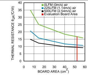
Figure 31. Package Thermal Resistance  $R_{\theta JA}$  4 Layer PCB With 1-oz Copper
