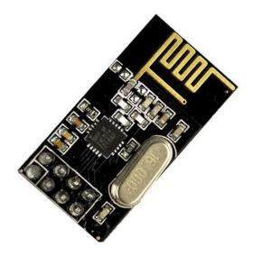
This module only different to <u>nRF24L01</u> is added a **250Kbps data rate**, which uses the newest 2.4GHz transceiver from Nordic Semiconductor nRF24L01+. This transceiver IC operates in the 2.4GHz band and has many new features! Take all the coolness of the nRF2401P and add some extra pipelines, buffers, and an auto-retransmit feature.
