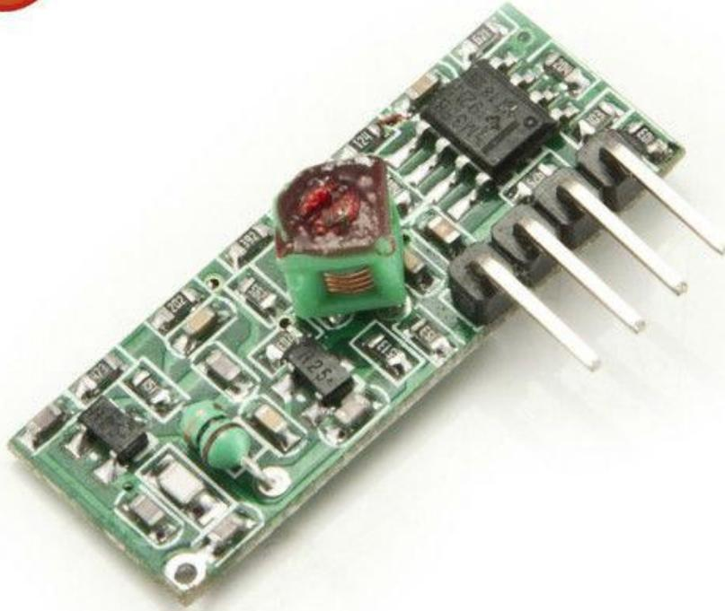
ZR-3A small size RF Super-regeneration Wireless Receiver Module 315MHZ/433MHZ
