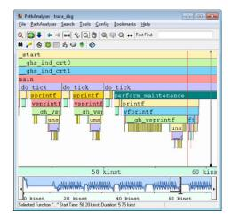
An invaluable part of the TimeMachine tool suite, the PathAnalyzer provides a view of your application's call stack over time. Click for larger view
