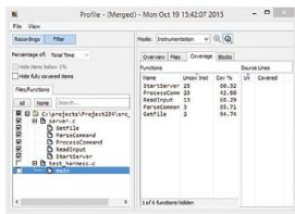
The Profiler's interface streamlines analyses, showing how often and for how long different tasks, functions, instructions, etc were called so you can pinpoint where to target optimization and testing efforts. Click here for a larger view.
