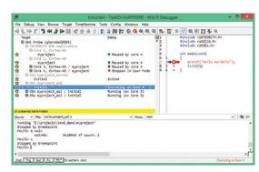
MULTI's synchronous run control halts all cores in a multicore system simultaneously. This enables you to debug one core without worrying that operations running on another core will affect shared memory. Click here for a larger view.
