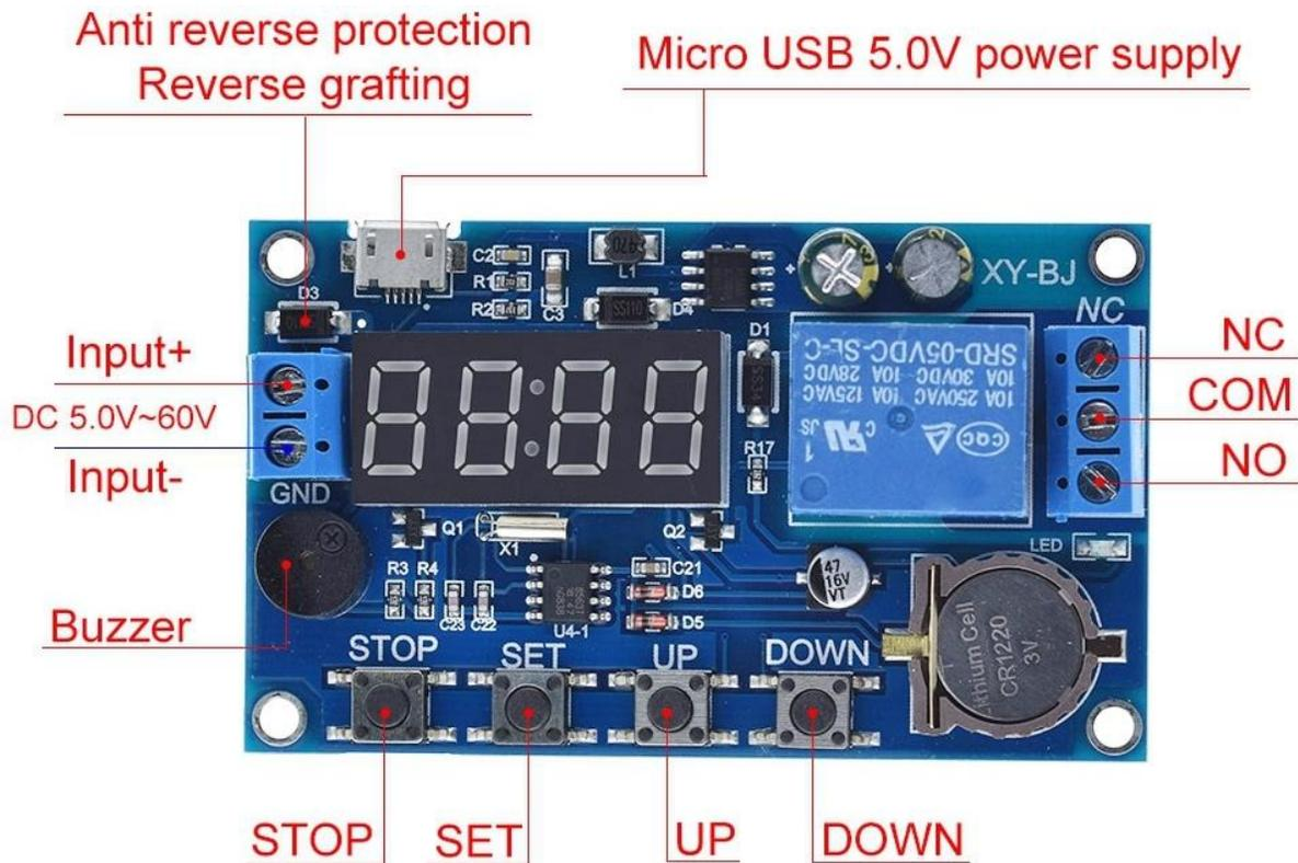
**Real-time relay Timing and clock synchronization
