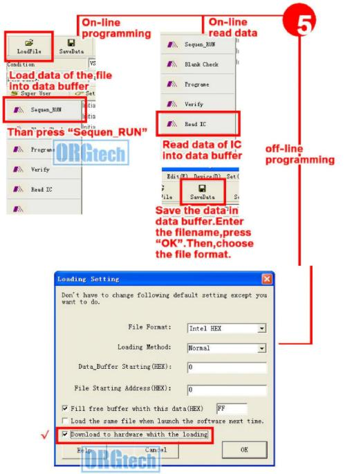
Off-line programming: If you have a file or you can read the data of chips and save, load the file, you should see the dialog box above. Check the "Download to hardware", and then, you can pull out the USB to do off-line operations.
