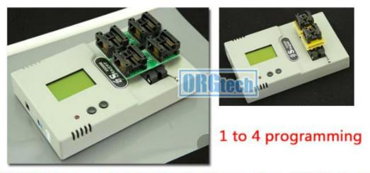
VSD8000 can program 4pcs IC at one time if you use the suitable IC adapter. This universal programmer can works as a production programmer.
